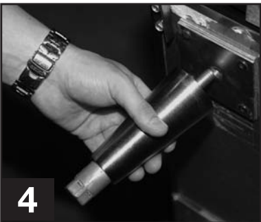
4 Thread leg into cabinet bottom frame rail.
